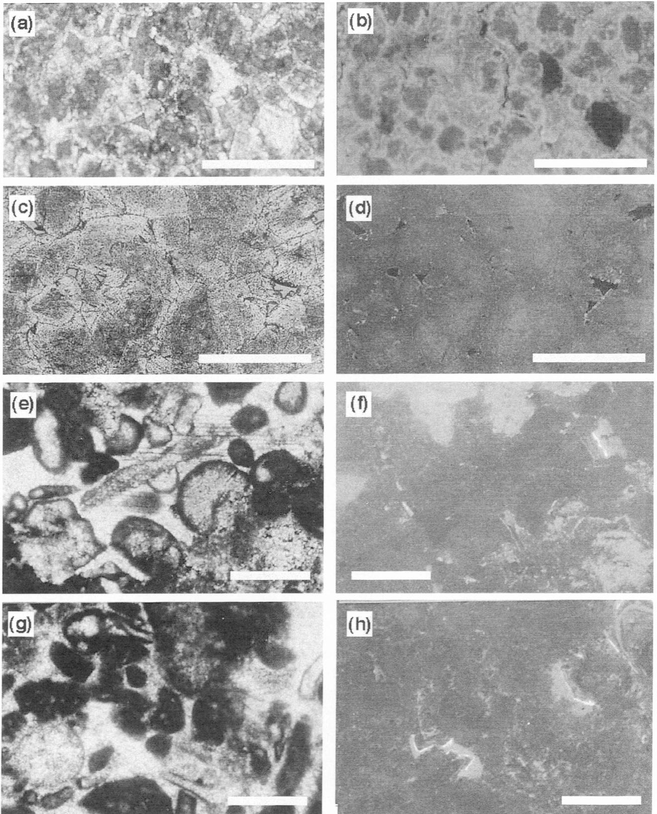
Fig. 6. Textures of optical microscopic (on the left hand) and cathodoluminescence (CL) views (on the right hand) of limestone and dolostone of units 1 and 2. All scale bars are 1 mm. (a, b) Partly dolomitized grainstone (K-10; unit 1). (c, d) Coarse dolostone (K-17; unit 2). (e, f) Peloidal grainstone (K-21; unit 2) showing banded cements. (g, h) Peloidal grainstone (K-25; unit 2) with cements showing clear zonation of CL intensity.
