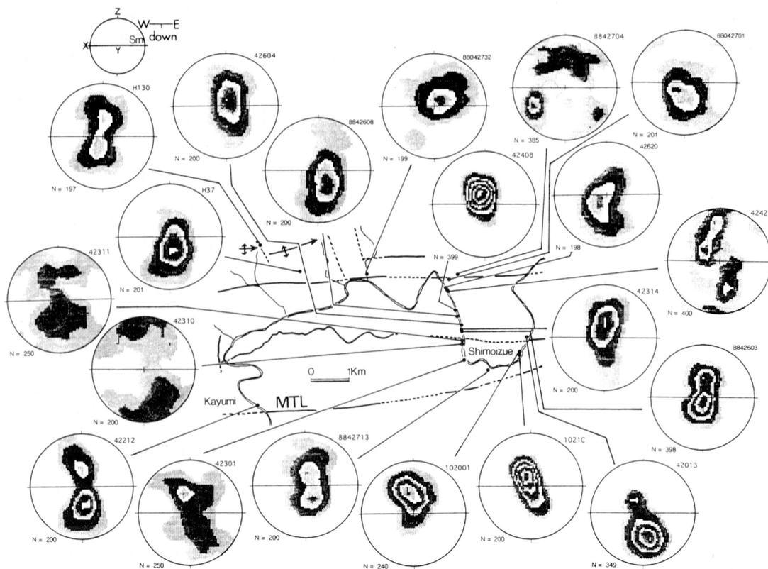
Fig. 10. Quartz c-axis fabrics in the southern part of the Kayumi district. Contour interval:  $2\sigma$  (Kamb method). X, Y and Z are maximum, intermediate and minimum principle axes of the finite strain respectively.
