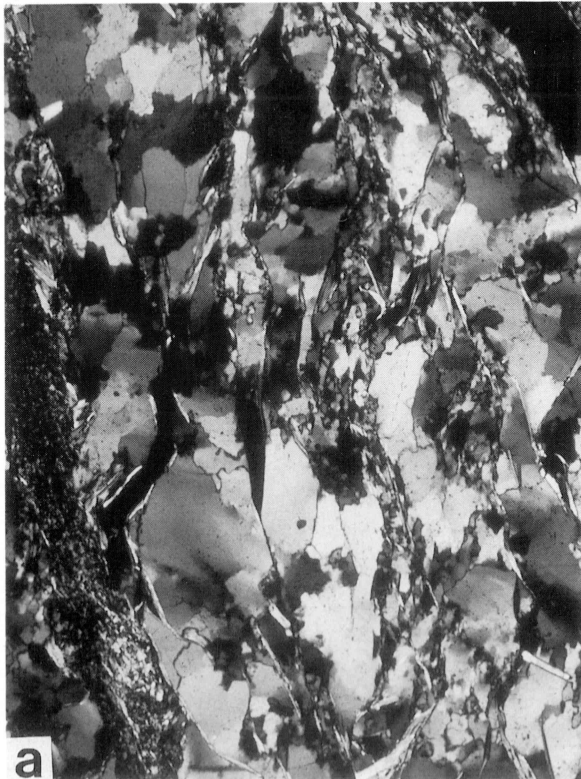
Fig. 11. Minute grains dynamically recrystallized along grain boundaries of quartz in quartz-rich layers of a Dh phase fold of flexural-slip type (Fig. 5). a) photograph of a quartz-rich layer bounded by R1 faults in limb, b) photograph of axial zone. Quartz grains are strongly elongated parallel to the axial plane.
