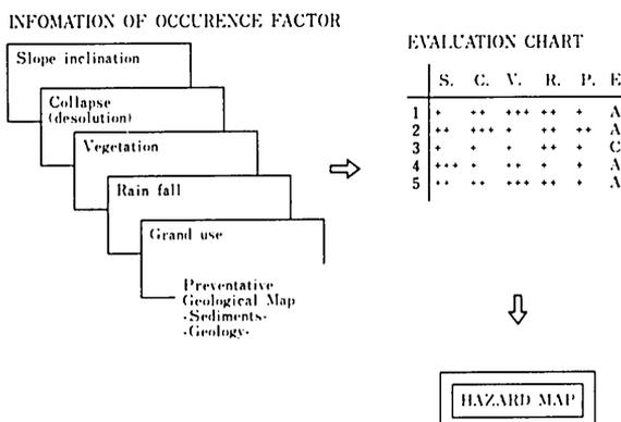
FIG. 26 Flow chart illustrating the composition process of the hazard map.
