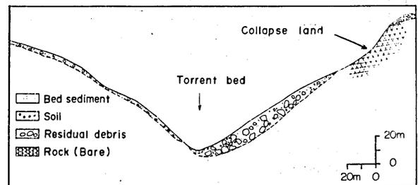
FIG. 2 Schematic cross-section of Gosukedani river basin illustrating the relationship between the residual debris and the torrent bed.
