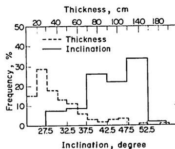
FIG. 12 Frequency distribution of inclination and thickness of the collapse at the Kure disaster of 1967 (by Aboshi et al., 1972)
