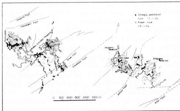
FIG. 19 Characteristic distribution of the strongly weathered rock (C1-C3 : circle) in Rokko district which is consisted of several fault blocks with steep fault scarps. Hard rocks of P1-P3 are represented by crosses. See Fig. 20.
