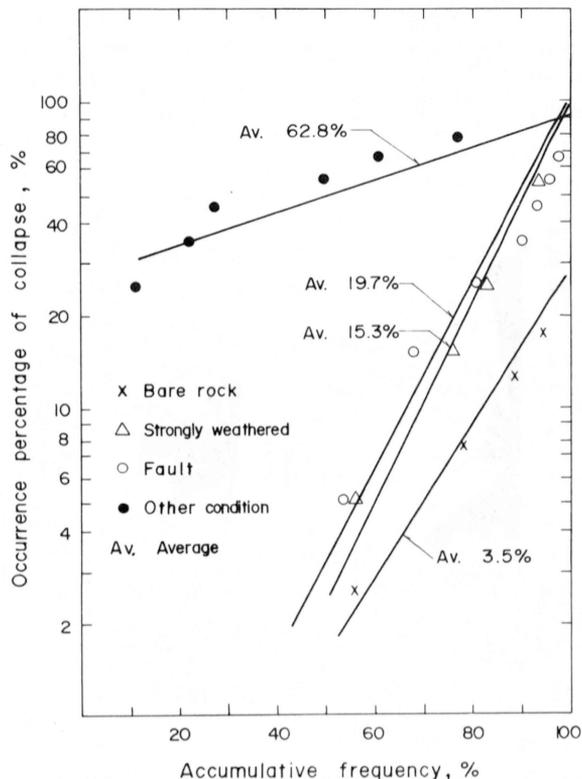
FIG. 18 Relation between collapse frequency and the geological factors.
