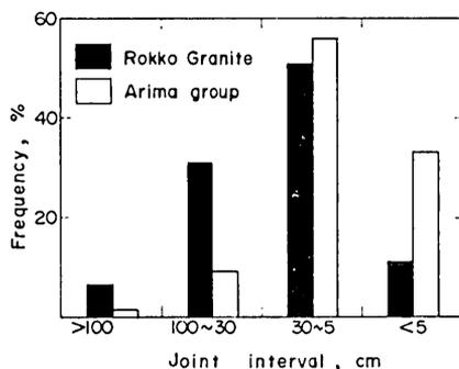
FIG. 13 Frequency distribution of joint interval observed in the granite and the rhyolitic tuff (Arima group). The data are those of in the catchment area of River Yamada, northwest of Mt. Rokko.
