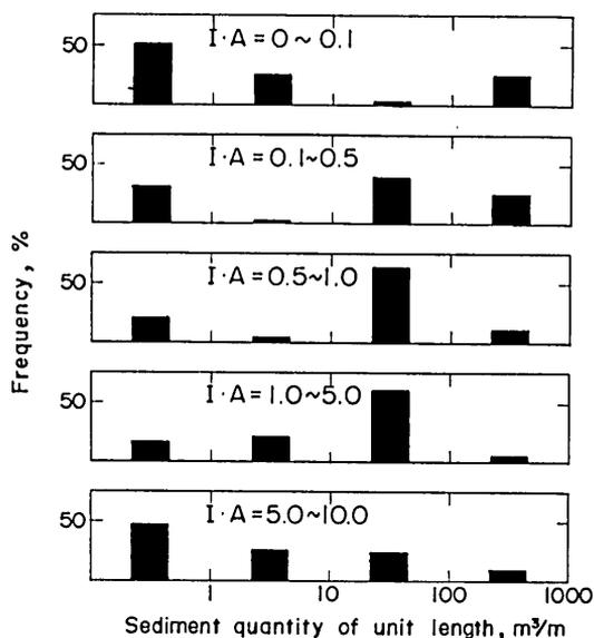
FIG. 22 Dependence of frequency distribution of movable sediments on the  $I \times A$ . I: bed inclination, A: Catchment area.
