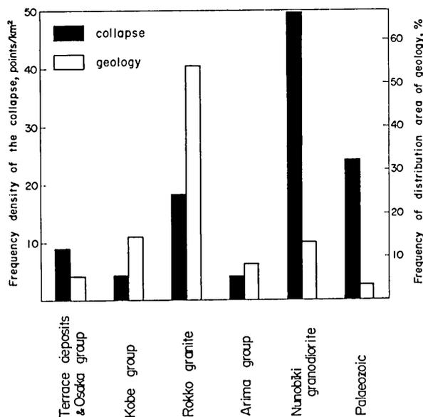
FIG. 11 Correlation of the frequency density of the collapse (solid pillar) and the distribution area of geology (open pillar).
