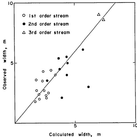
FIG. 5 Relation between the observed and calculated widths of S- II surface. The calculation was based on the Regime-theory related 100-year discharge.
