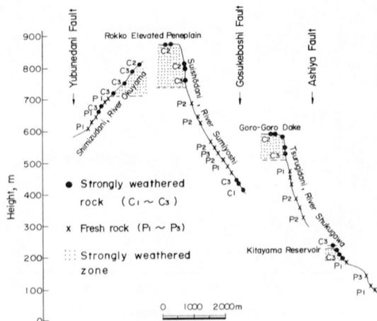
FIG. 20 Schematic cross-section profile of the districts shown in Fig. 19. See text.
