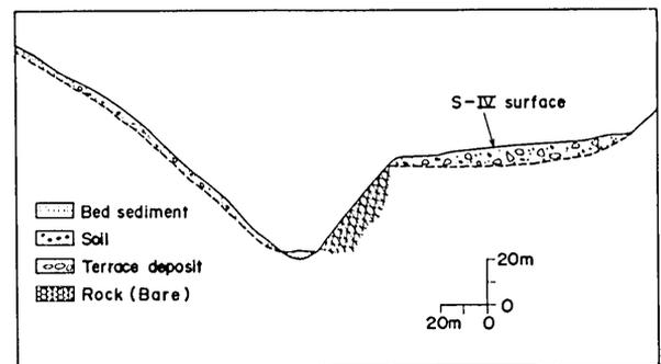
FIG. 7 S-IV surface (terrace deposits) developed at relatively higher level compared with that of the torrent bed (see text).
