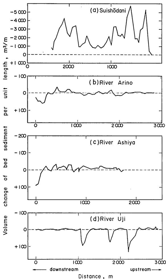
FIG. 21 The volume change of the bed sediments along several rivers at the Rokko disaster of 1967. The dotted line separates the discharge (above) and deposition (below). See text.
