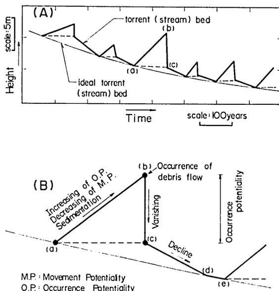
FIG. 23 Schematic illustrations of the movement and disaster potentialities.
