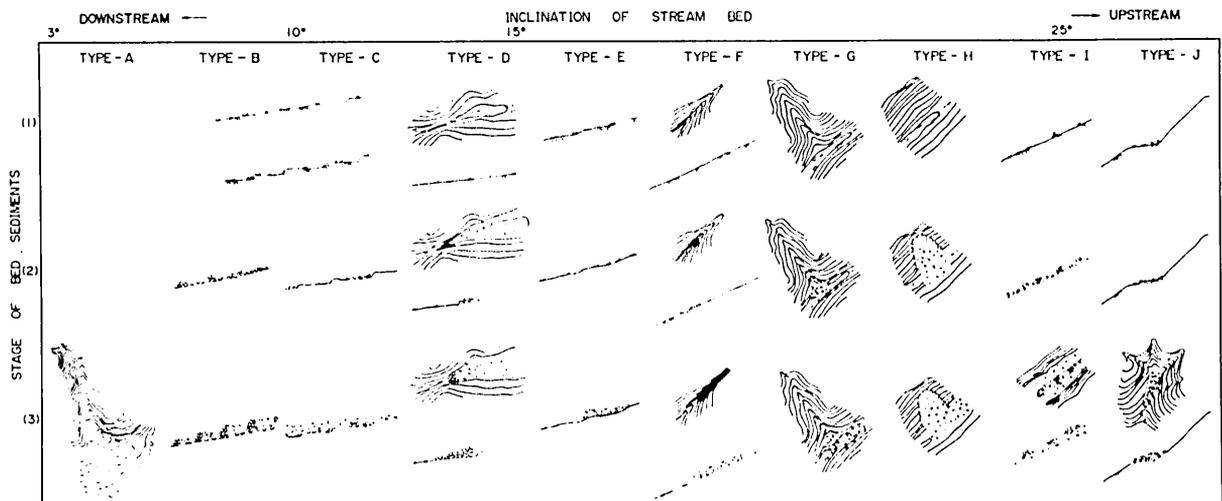
FIG. 8 Classification of the bed sediments based on the formation process and the geomorphological situation. Characteristics of each type are represented by both vertical and/or horizontal planes.
