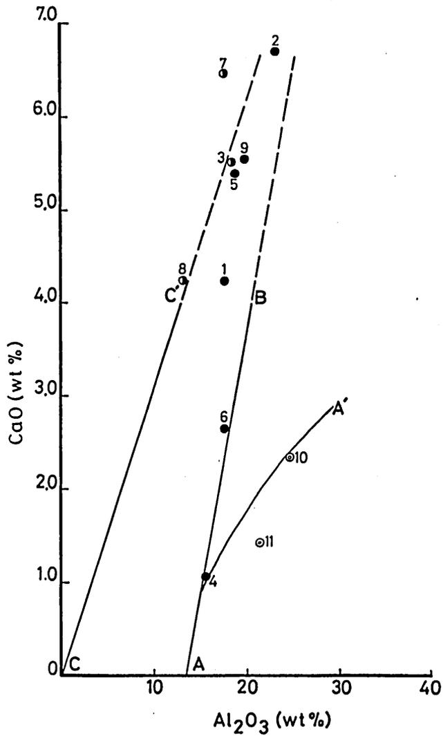
FIG. 5. The compositional distribution of metapelites in the Odori-River district. Double circles: sillimanite present, solid circles: no aluminium silicates (almost with muscovite), half open circles: hornblende or clinopyroxene present. The numbers attached to circles refer to the column numbers in Tables 1 and 2. The explanation for the curves is presented in the text. Dashed lines are extended by the author.
