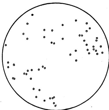
FIG. 4. (0001) pole diagram of calcite porphyroblast in the specimen 3.
