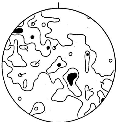
FIG. 1. (0001) pole diagram of matrix calcite in the specimen 1. contours: 4-2-1%
