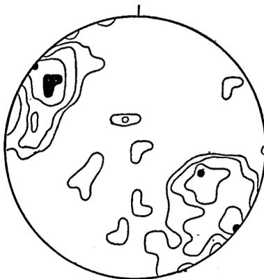
FIG. 2. (0001) pole diagram of calcite porphyroblast in the specimen 1. contours: 8-4-2-1%
