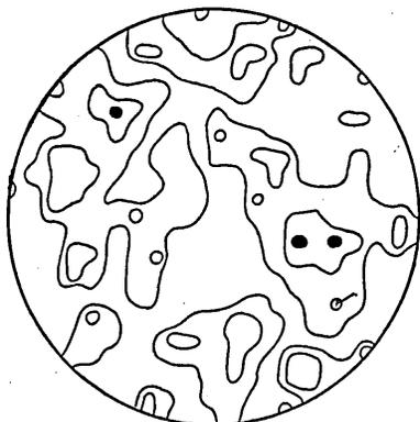
FIG. 3. (0001) pole diagram of calcite porphyroblast in the specimen 2. contours: 4-2-1%
