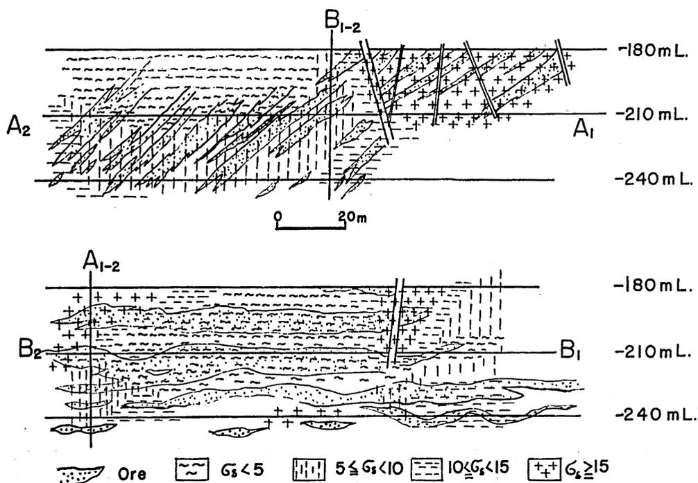
FIG. 26. Schematic profile sections of the lower ore deposit along  $A_1 \sim A_2$  and  $B_1 \sim B_2$  drawn in Figs. 23, 24 and 25.
