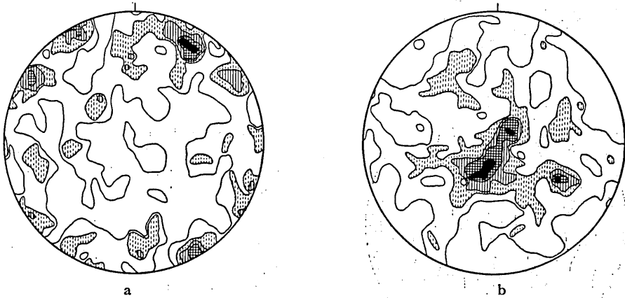
FIG. 6. Orientation diagrams for light-coloured clinopyroxene in Section GY 59 VIII 18-5. 200 grains existing outside the large grains of black clinopyroxene were selected.
