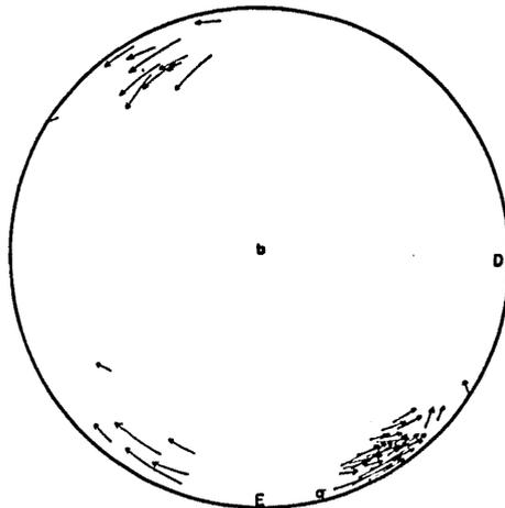
FIG. 5. c-Axes of lamellar crystals (point of arrow) and those of host crystals (end of arrow).
