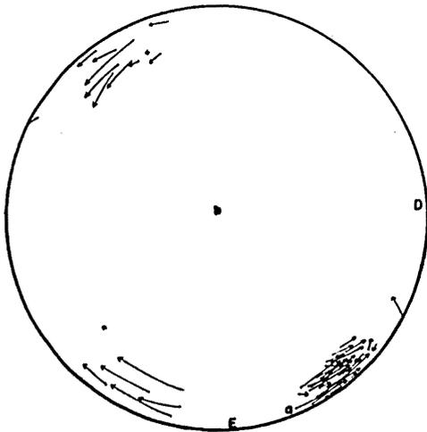
FIG. 3. Poles of lamellae (point of arrow) and c-axes of host crystals (end of arrow).
