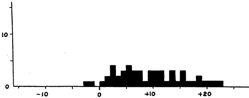
FIG. 6. Histogram showing the variation in the angle between the c-axis of host crystal and the pole of lamellae.
