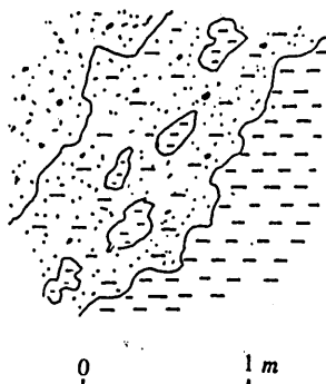
FIG. 8. Sketch showing the mode of contact between pyrite ore and acidic tuff. The contact is gradual, and there are many replacement remnants of acidic tuff in disseminated ore.
