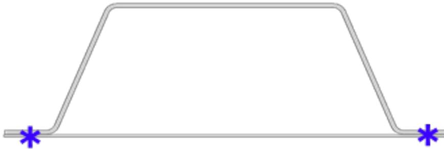
Fig.65 Conventional B-pillar cross-sectional shape.
