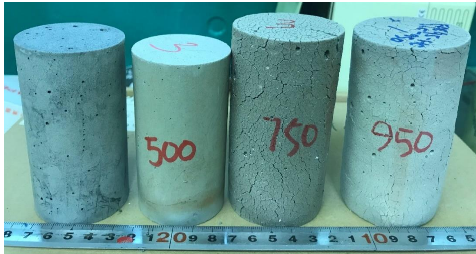
Figure 4.4 Visual appearance of unexposed and exposed geopolymer containing 45% GGBS
