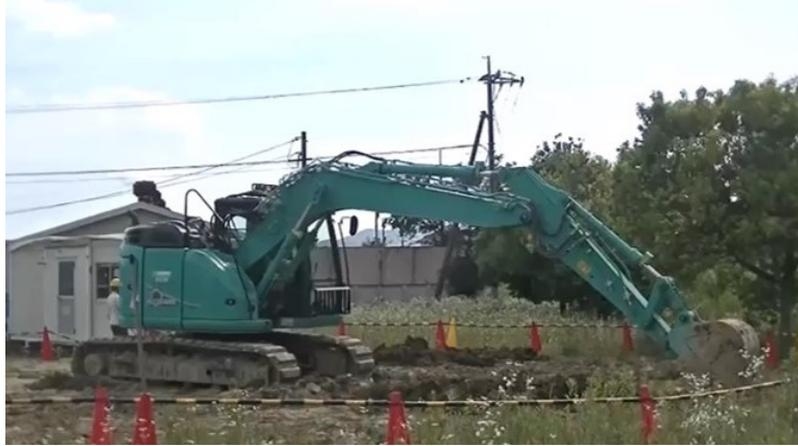
Fig. 2.4: Real excavator (SK135SR-5, Kobelco Construction Machinery).
