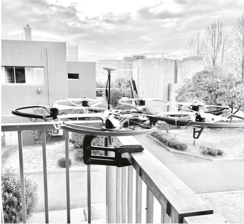
**Figure 1.2: Multicopter with simple underactuated device can perch on veranda easily for delivery, security monitoring, etc.**
