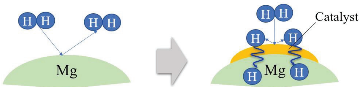
Figure 1.6 Shows the catalysts spread on Mg surface provided the dissociation of the hydrogen molecule
