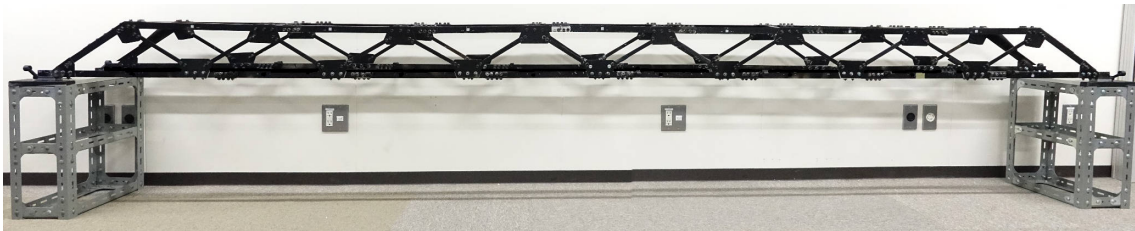
Figure 2.10: Truss bridge model (corner cube prism experiment).
