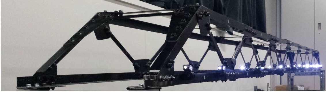
Figure 2.1: Test truss structure with LEDs attached on a single lower chord of the truss.
