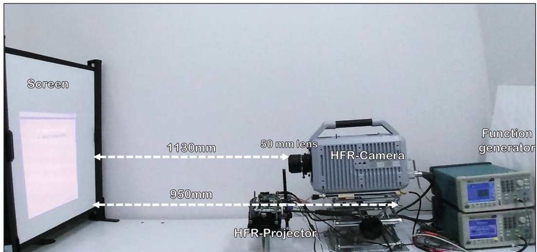
Figure 5.24: Overview of the HFR projector-camera system.
