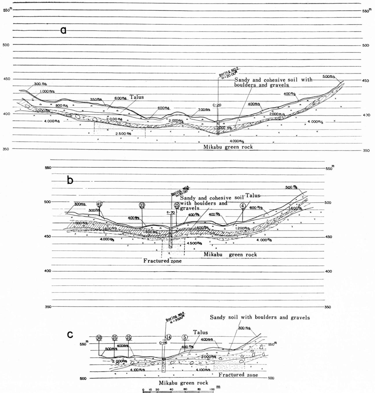
FIG. 7. a : Section on the lowest level along the slope at Nakaguroiwa.
