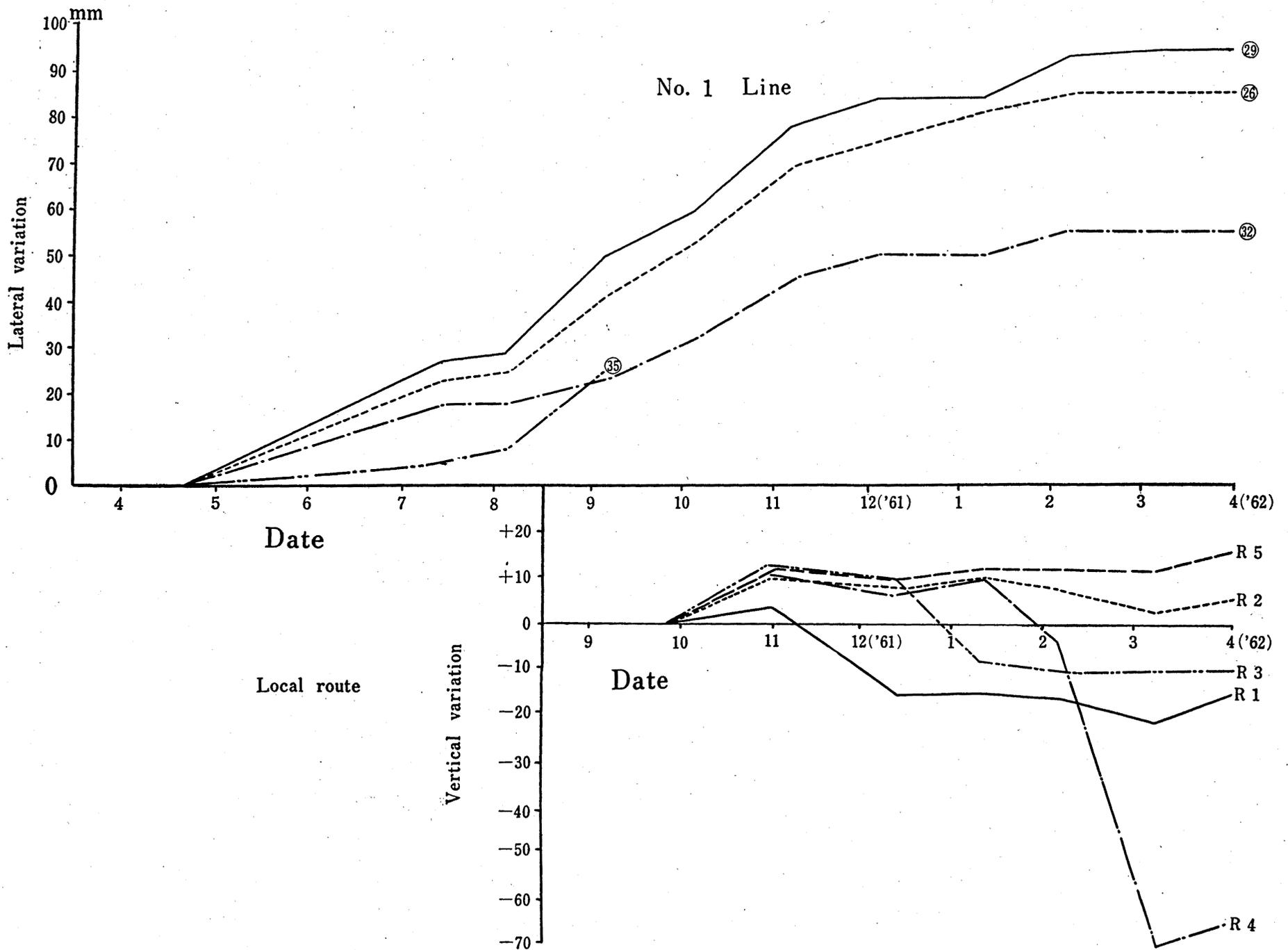
FIG. 10. Lateral and vertical movements observed in the Kassen area.
