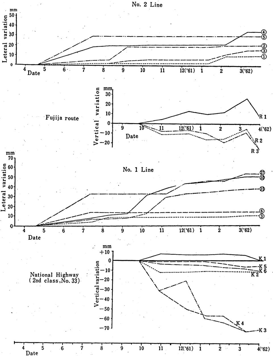
FIG. 12. Lateral and vertical movements observed in the Kassen area.
