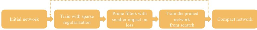
FIGURE 3.1: Flow-chart of the feature-wise filter pruning procedure.
