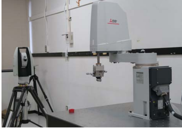
Figure 8: Tracking interferometer measurement setup.
