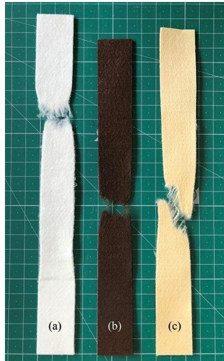
Figure 2.3 Appearance of filter media: (a) original; (b) exposed to Gas I (NO 2 + heat) for 200 h; and (c) exposed to Gas II (heat) for 200 h.
