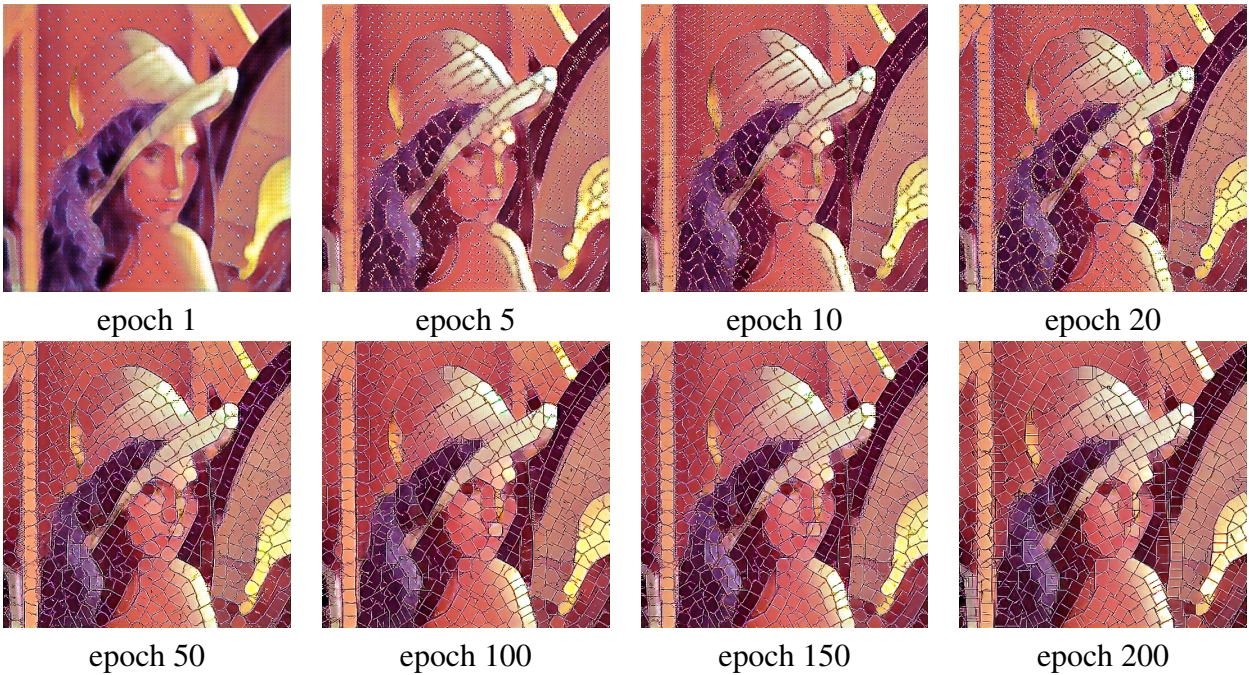
Figure 4.13: The output images of the generator during the training. At epoch 1, the original image still appears as it is. At epoch 50, tiles become visible, however, the edges of tiles are thin. At epoch 200, tiles become clearly.
