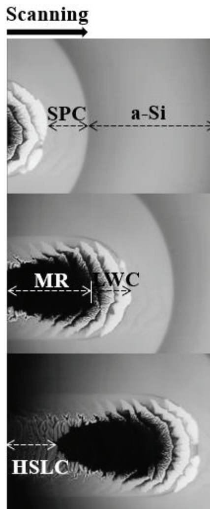
Fig.1.5. HSC snapshots of Si film taken by HSC during \mu -TPJ irradiation. \mu -TPJ conditions were f_{Ar} = 1.6 L/min, P = 1.12 kW, v = 1500 mm/s, d = 1.0 mm, ES = 2.0 mm.
