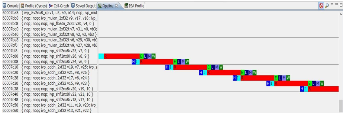
Figure 59. Pipeline Analysis View of Xtensa Xplorer [121].
