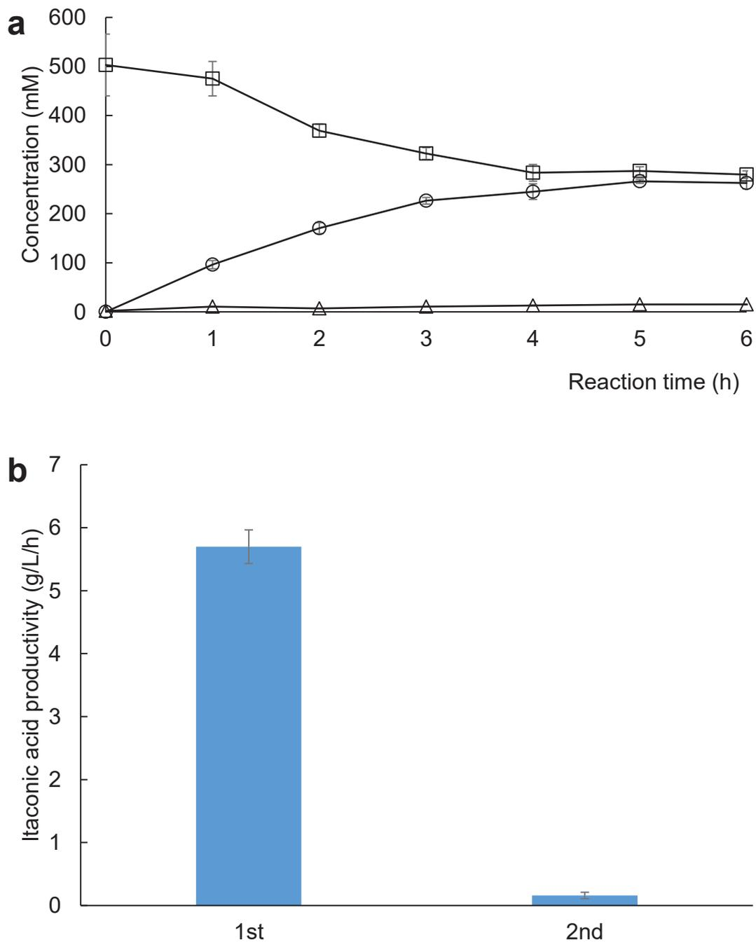
Fig. 3.9 Time-profile of itaconic production at 50 °C by recombinant *S. livingstonensis* Ac10 cells after heat permeabilization (a). Rectangle, citric acid; circle, itaconic acid; triangle, *cis*-aconitic acid. Itaconic acid productivity of recycled cells (b). Error bars represent the standard deviation of the mean (n = 3).
