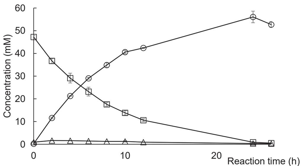
Fig. 3.7 Time-profile of itaconic acid production by heat-permeabilized *S. livingstonensis* Ac10 cells at 45°C for 15 min. Rectangle, citric acid; circle, itaconic acid; triangle, *cis*-aconitic acid.
