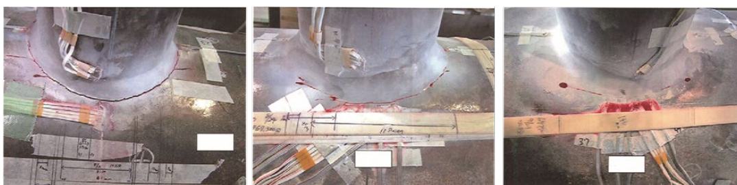
Fig. 3-2 Overall view of fractured test specimens [(a) \rho = 3 mm, (b) \rho = 6 mm, (c) \rho = 11 mm]
