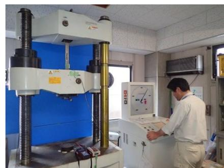
Fig. 4.6 Universal testing machine
