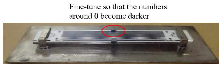
Fig. 7.10 Installation completion of strain visualization device
