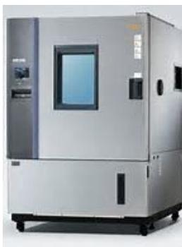
Fig. 3.9 Thermostatic chamber
