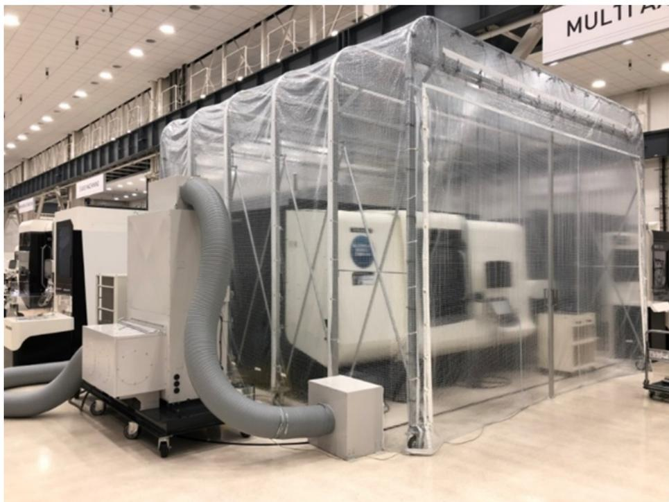
図 3.11: Movable temperature variable booth and air conditioner
