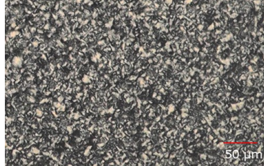
Fig. 5-6 A polarized light microscopic image of cocoa butter crystal containing AMF and lecithin before the thermal processing
