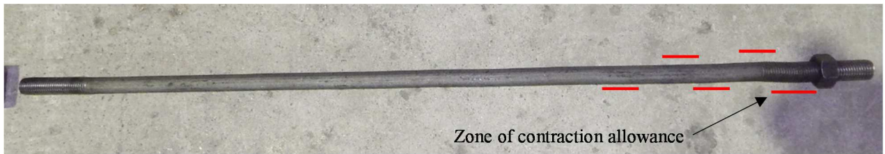
Figure 2.24 Lower core bar deformation after loading test (T-1)
