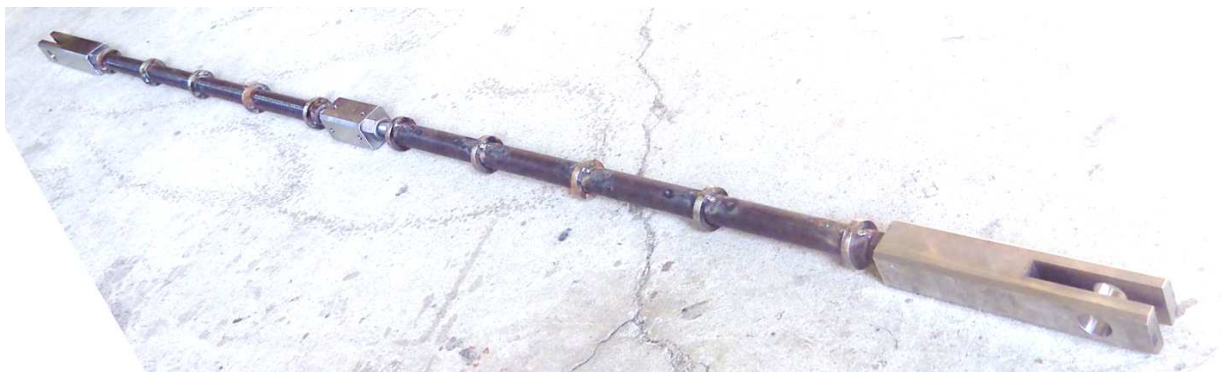
Figure 2.9. Built-up specimen T-1: Core bars, central and end couplers, and inner tubes (prior to incorporating the outer tube)
