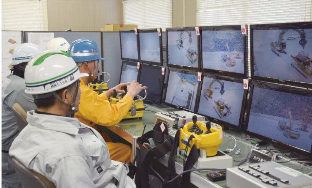
Fig. 1.2: Currently mainstream teleoperated hydraulic excavator system[27].
