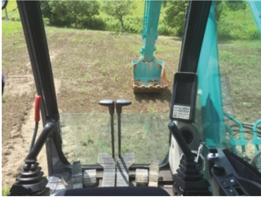
Fig. 2.2: Boom of hydraulic excavator obstructs operator's visibility.
