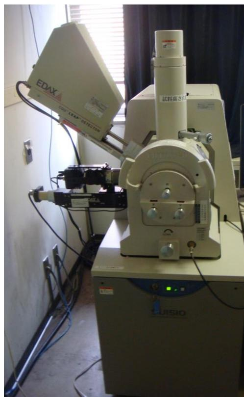
Fig.2-3 Electron BackScatter Diffraction device.
