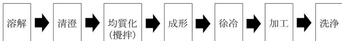
Fig. 1-3. Manufacturing process of glass.
