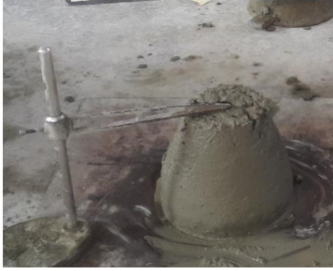
a) Slump test
