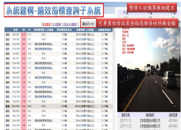
Fig. 7-11 Reconstruction Methods and Estimated Costs for Sections with Abnormal Indices
