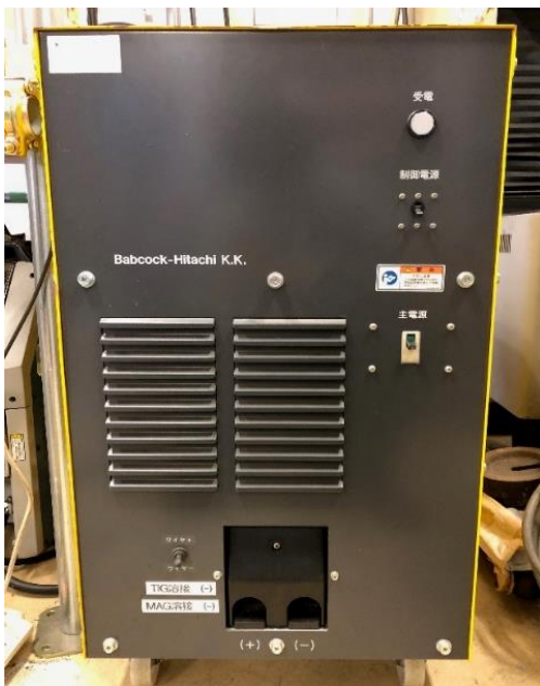
Fig. 5.5 Hot-wire power source.
