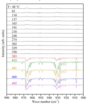
Figure 4 IR spectra of outlet gas from column with Li<sub>17</sub>Sn<sub>4</sub> alloy at different temperature
