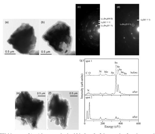
Figure. 3 TEM images of (a, e)the as-synthesized Li<sub>17</sub>Sn<sub>4</sub>, (b, f)the sample after nitrogenation, and (c, d) electron diffraction patterns, and (g) results of EDS analyses for spot 1-2 before and after the nitrogenation
