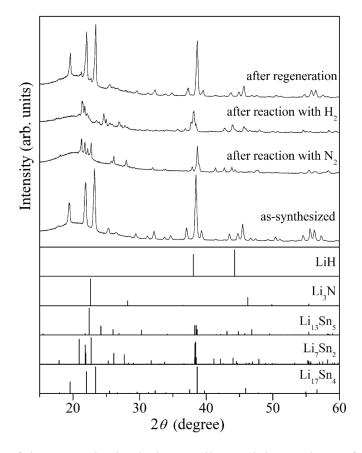
Figure 2 XRD patterns of the as-synthesized Li<sub>17</sub>Sn<sub>4</sub> alloy and the products after the reactions.
