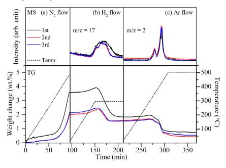
Figure 1 TG-MS profiles of Li<sub>17</sub>Sn<sub>4</sub> under 0.1 MPa of (a)N<sub>2</sub>, (b)H<sub>2</sub>, and (c)Ar flow conditions.
