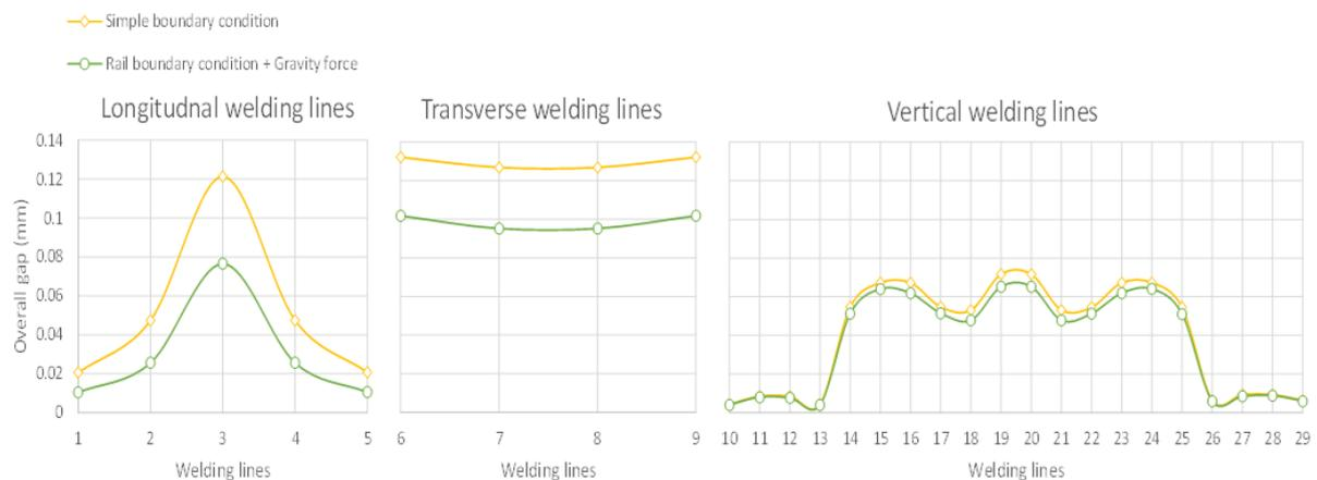
Figure 5.5 Total gap between the welding lines and plate, after welding each line
