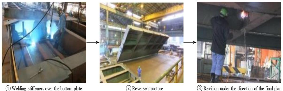
Figure 5.11 Welding work process of a hatch cover
