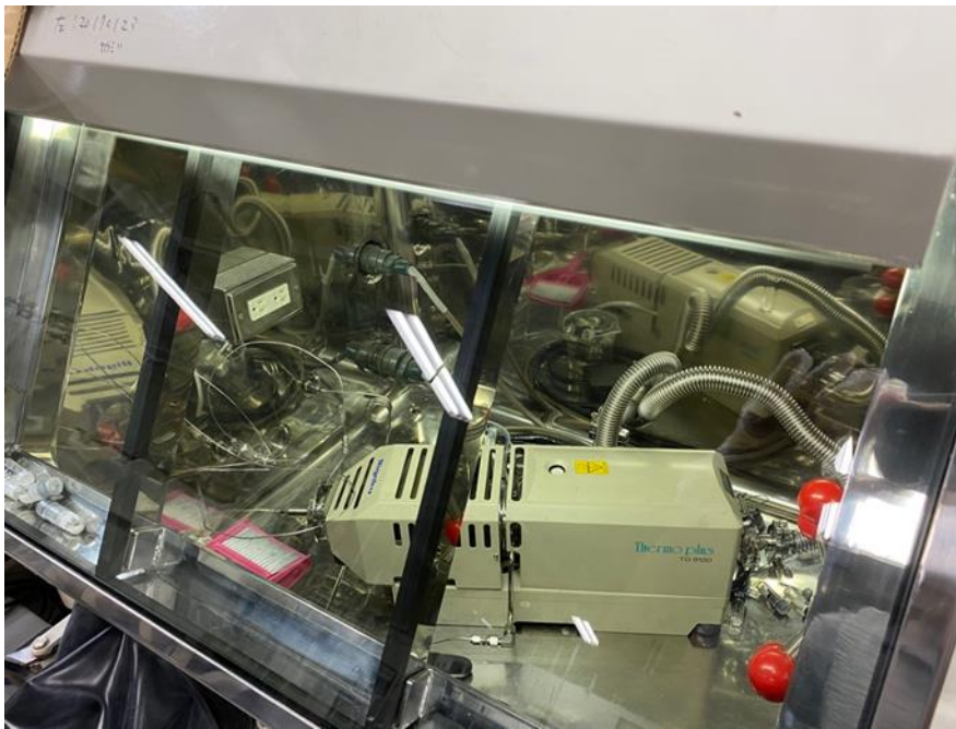
Figure 3.6 A picture of TG-DTA apparatus located in glove box.
