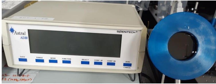
Fig. 125: Energy detector (calorimeter) used for measurement of laser-energy. The system is calibrated for 1064 nm radiation and reflections (~10%) occurring at the surface of the detection-head.
