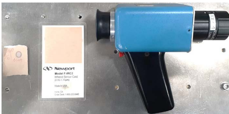
Fig. 221: Tools how to make the IR-beam visible. Thermal “burn”-paper (left), Phosphor-card (center), and IR-view (right). Thermal paper is useful to record the beam pattern, while the thermal paper is better used for alignment purposes. The IR-viewer can be used to visualize reflections, which can be useful for alignment.
