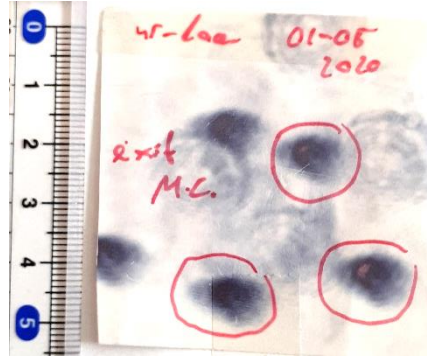
Fig. 174: Burn patterns of the ns-laser near the experimental chamber.
