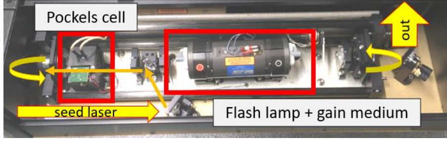
Fig. 120: Inside of a Q-switch-based Nd:YAG laser with an active shutter (Pockels cell). A seed laser beam is injected via a mirror and a polarizer. From there, the light passes through the Pockels cell and is reflected at the left mirror. Then the light passes through the whole system (Pockels cell, polarizer, laser medium) until it is reflected back at the right mirror. Each round trip, the energy carried in one pulse increases exponentially. The gain saturation is achieved after \sim 185 \mu\text{s} . When the Pockels cell is activated, the accumulated giant pulse leaves the cavity and the Nd:YAG-crystal can regenerate for the next shot. Stable operation is achieved after a warm-up time of \sim 30\text{-}60 \text{ min} .
