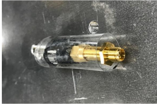
Fig. 141: Photodetector AXUVHS5DS for measurement of X-ray pulse duration.
