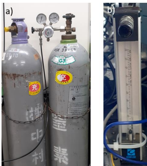
Fig. 97: (a) Gas bottles of nitrogen ( \sim 15 MPa) and (b) flow controller. The pressure regulator scales the high pressure in the bottle down to \sim 1 MPa. From there, the flow controller is connected and provides up to 5 L/min. gas-feed to the experimental chamber.
