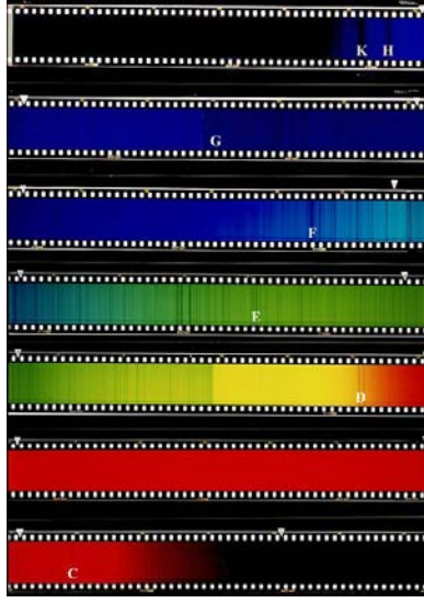
Fig. 77: Fraunhofer-lines observed with 25cm Coronagraph, Norikura Solar Observatory & Solar Optical Telescope, Hinode (Solar B) [150]. The famous sodium-doublet D consists of two lines at a center wavelength of \sim 589.29 nm originating from a fine-structure splitting.
