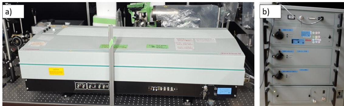
Fig. 123: (a) The commercial Nd:YAG laser. (b) The control unit, power unit, capacitor bank, and cooling unit.
