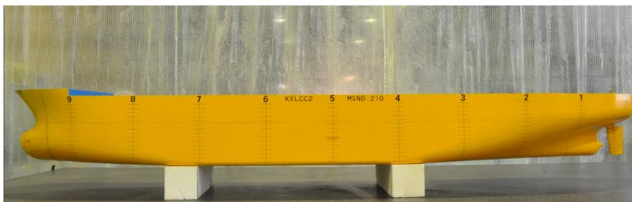
Fig. 3.2: Side profile of a KVLCC2 model
