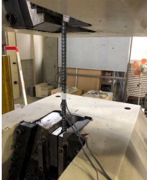
Figure 2.2.3. Coupon of a steel bar under the tensile strength test.
