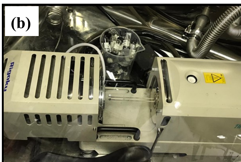
Fig. 3-9: (a) Rigaku, TG8120 connected to a mass spectrometer (MS, Anelva, M-QA200TS) glove box, (b) TG-DTA instrument inside the glove box
