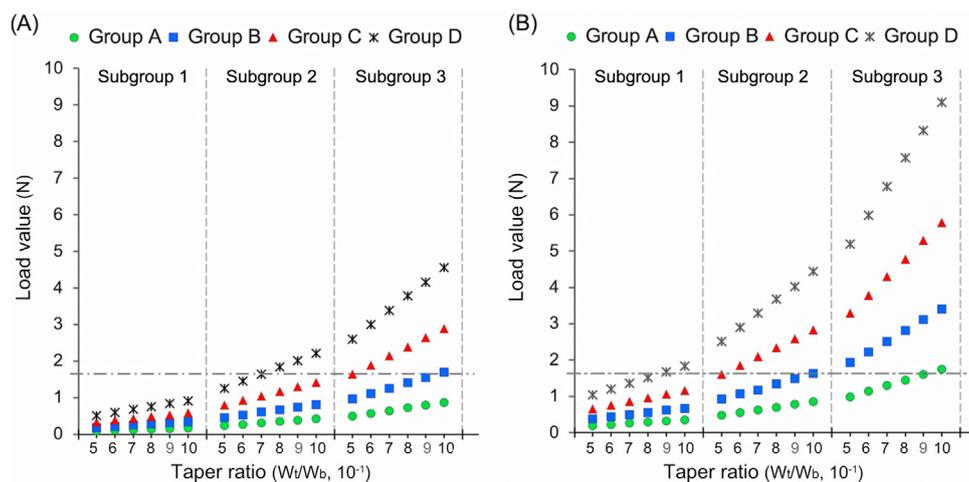
**Fig. 2.** Load values when constant displacements of (A) 0.25 mm and (B) 0.50 mm were applied to the 3D models. The horizontal dashed line represented the lowest acceptable retentive force (1.6 N) of RPDs.
