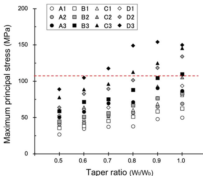
**Fig. 3.** Maximum principal stress of each 3D model when load measured at constant displacement of 0.50 mm.
