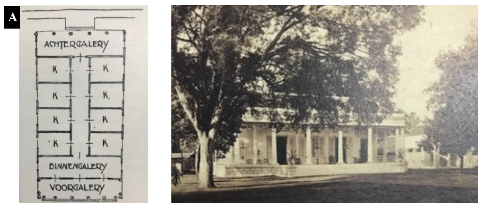
Fig4.43 The Dutch Indies Empire houses 23) (A. Typical floor plan, B. Façade)
