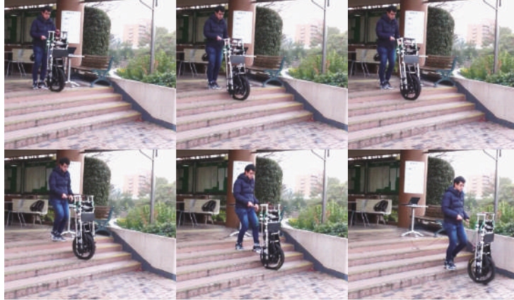
Figure 3.26: Snapshots of a single-wheeled robot descending stairs.
