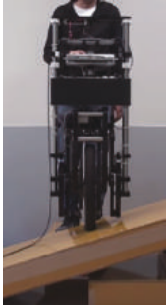
Figure 3.20: Snapshot of the robot stabilizing on a lateral slope with an angle of 16^\circ .
