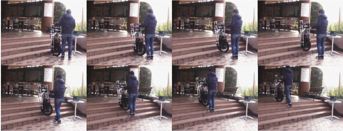
Figure 3.24: Snapshots of a single-wheeled robot ascending stairs.
