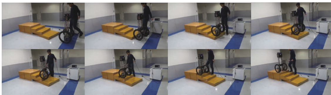
Figure 2.19: The snapshots of the robot climbing a curved staircase.
