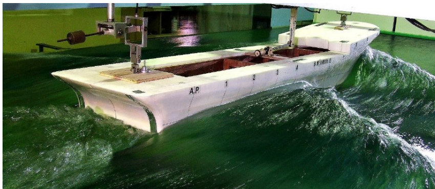
Photo 5-3 Wave pattern of prototype saury fishing vessel. - V_s = 11 knot, F_n = 0.388 -
