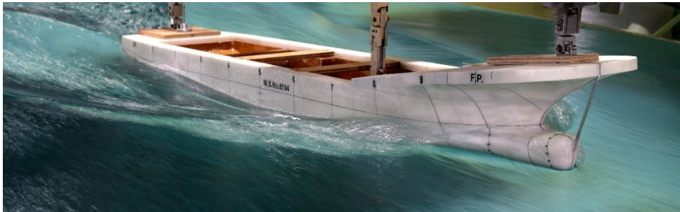
Photo 5-12(1) Wave pattern from fishing port of improved type set net fishing boat with propeller guard. - V_s = 12\text{knot} , F_n = 0.407 -
