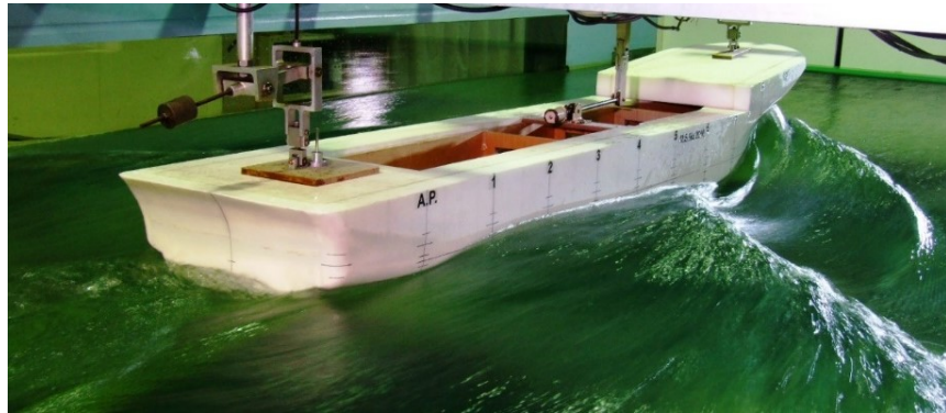
Photo 5-4 Wave pattern of improved type saury fishing vessel. - V_s = 11 knot, Fn = 0.371 -
