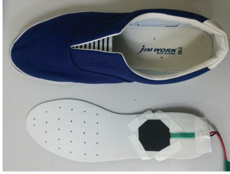
Fig. 2.11: FSR sensor fixed to heel portion of the shoe to detect stance phase of the gait cycle.
