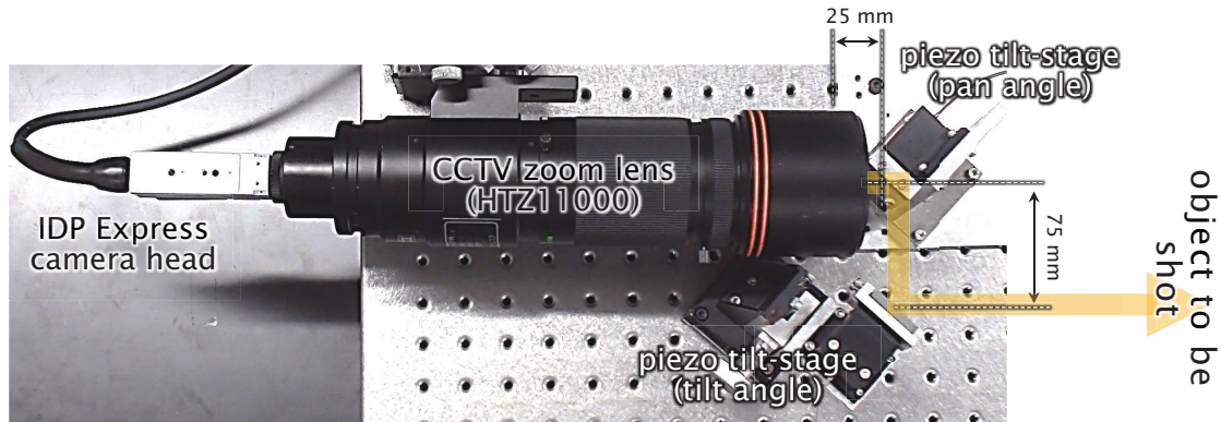
Figure 4.1: Overview of motion-blur-free video camera system using a piezo mirror.
