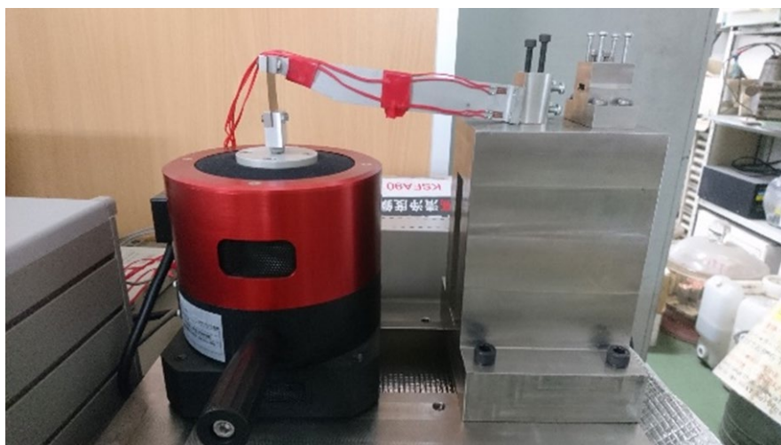
Fig. 2-2 Photo image of plane bending fatigue tests machine.
