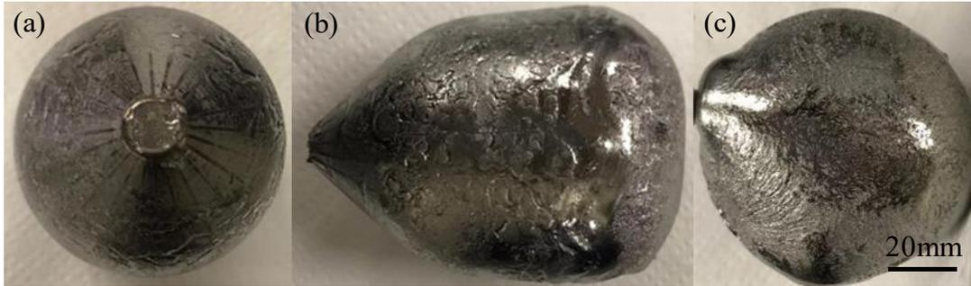
Fig. 2-8 The images of ingot produced by CCLM, (a) bottom, (b) side and (c) top views.
